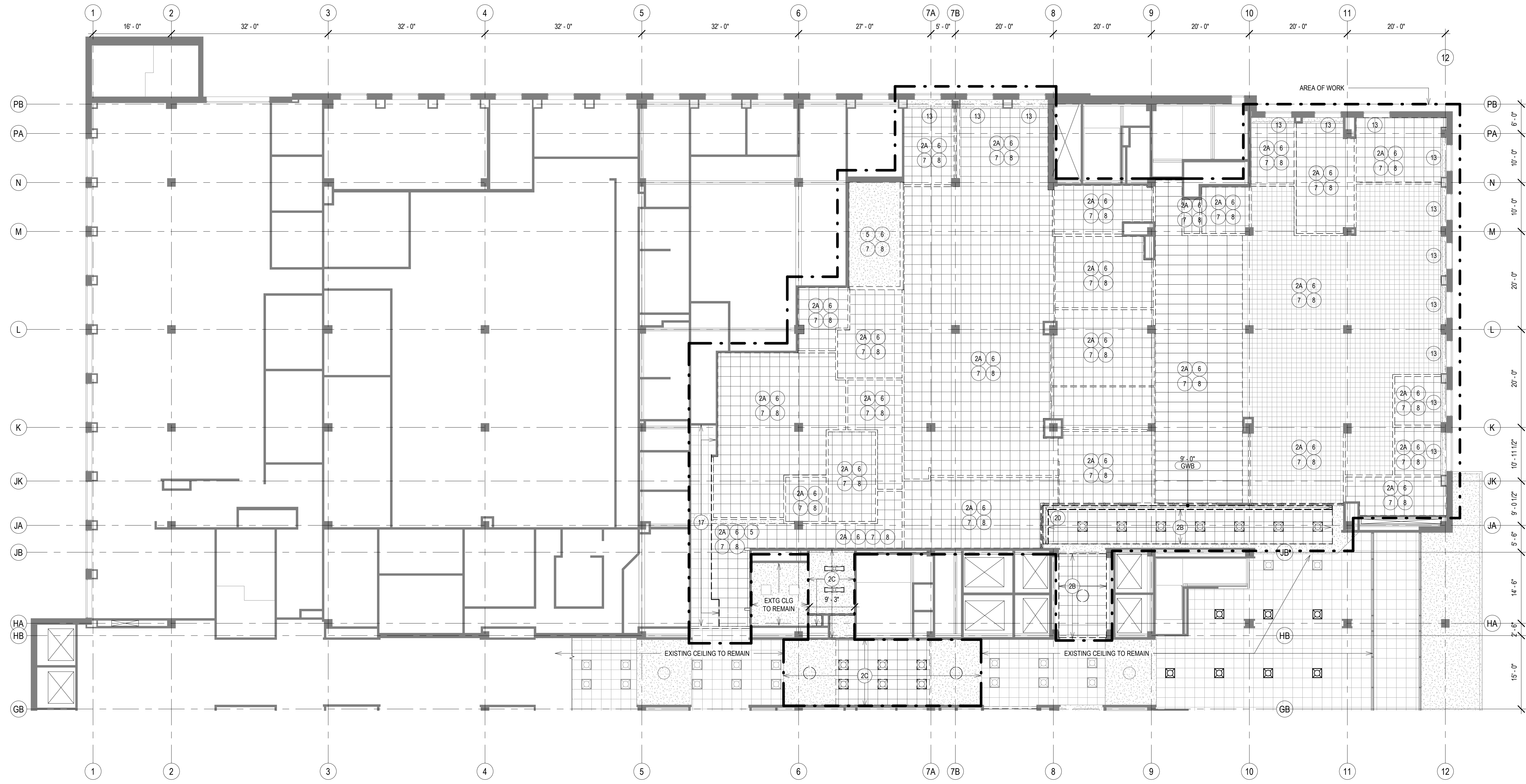
1 DEMOLITION REFLECTED CEILING PLAN - LEVEL 01 - OVERVIEW - NORTH Scale: 3/32" = 1'-0"
